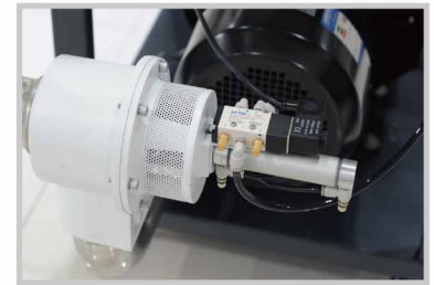
Vacuum breaking valve
