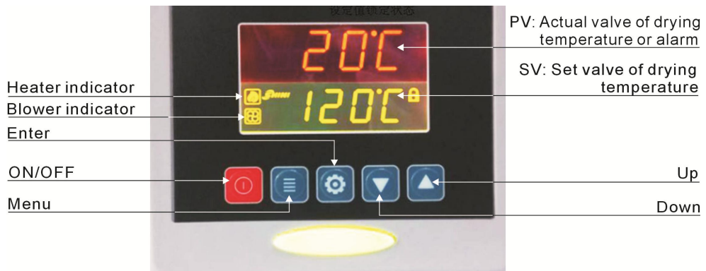
Picture 4-1: Control Panel
