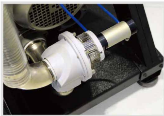
Vacuum breaking valve
