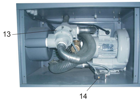
Picture 3-5: Conveying Blower
