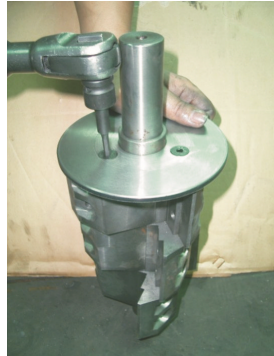
Picture 6-11: Installation of material fender
