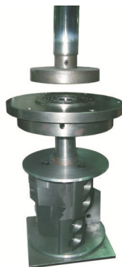
Picture 6-12: Installation of bearing block and bearing
