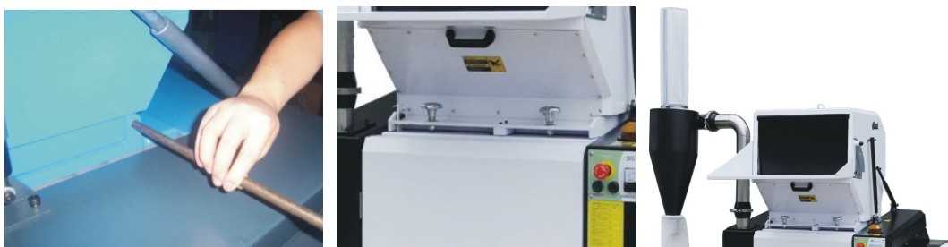
Picture 6-16: Installation of rotary blade and fixed plate (3)
