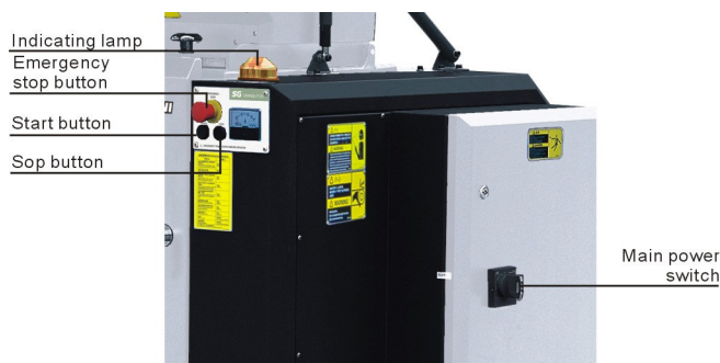
Picture 2-2: Emergency stop switch
