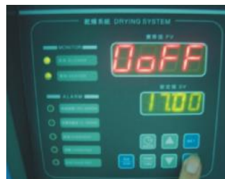
Picture 4-2: Intermittent Drying Setting-Chart 2
