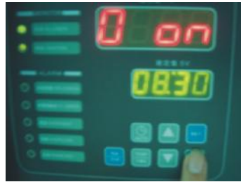
Picture 4-1: Intermittent Drying Setting-Chart 1
