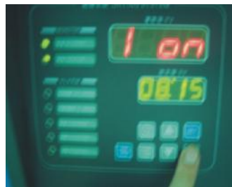
Picture 4-4: One-week Automatic Start / Stop Timer-Chart 1
