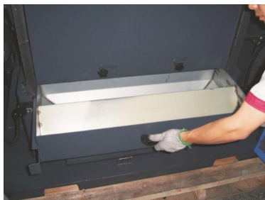
Picture 6-13: Installation of Storage Box, Screen and Screen Bracket 5
