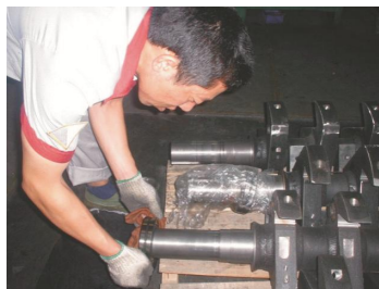
Picture 6-4: Installation of Bearing and Blade Rest
