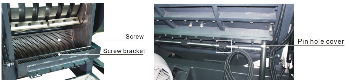
Picture 6-10: Installation of Storage Box, Screen and Screen Bracket 2
