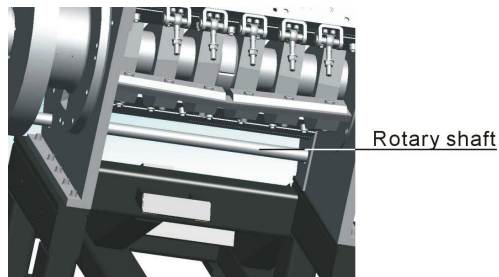
Picture 6-9: Installation of Storage Box, Screen and Screen Bracket 1
