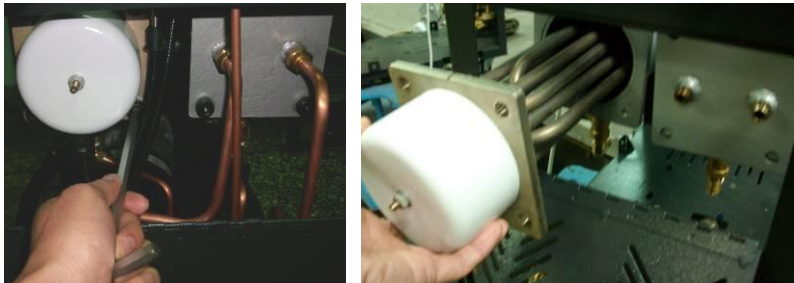
Picture 6-7: Pipe Heater 2
