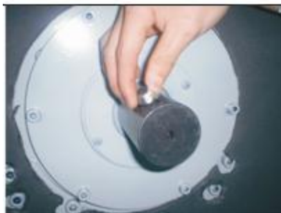
Picture 3-4: Installation of Belt and Belt Pulley 1
