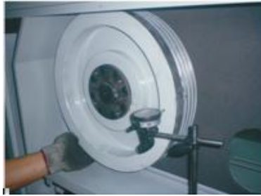
Picture 3-5: Installation of Belt and Belt Pulley 2
