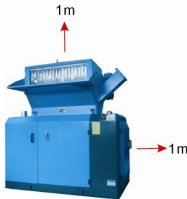
Picture 3-1: Installation Place
