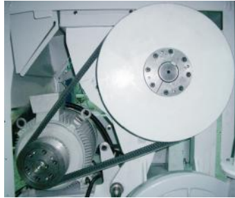
Picture 3-8: Installation of Belt and Belt Pulley 5
