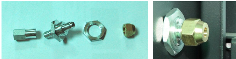
Picture 2-4: Copper joint assembly of original machine
