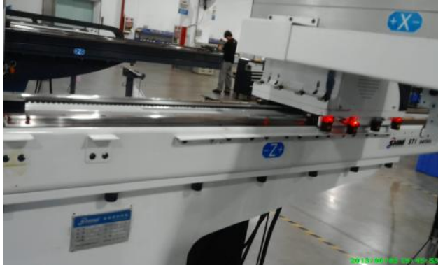
Picture 3-4: Outside IMM safety zone blocks after modified
