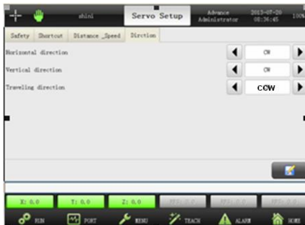
Picture 3-8: Direction After Modified
