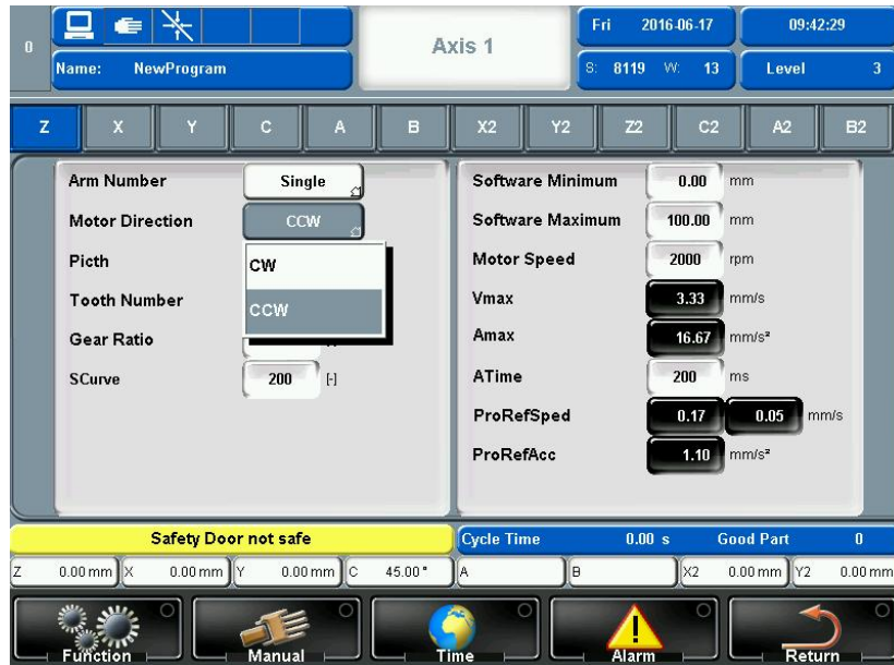
Fig.3-10: Servo motor direction before reversing
