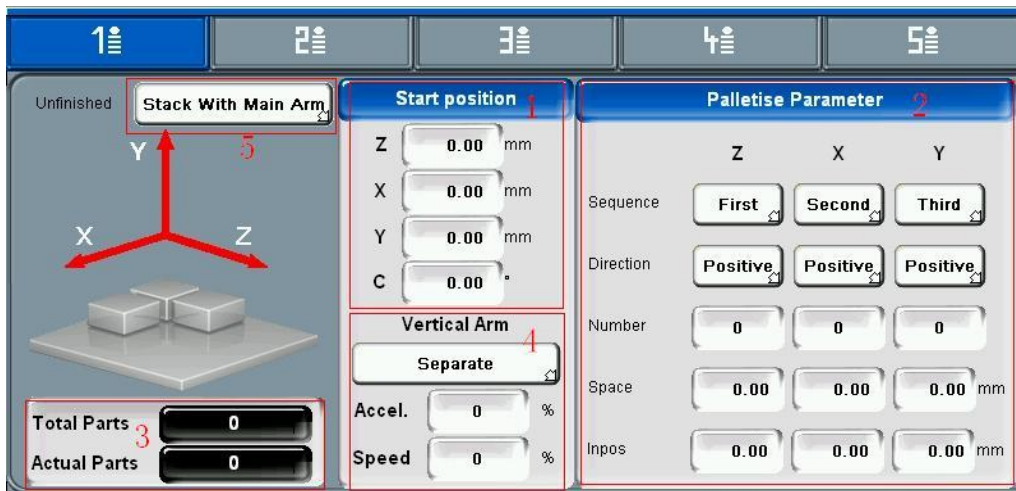
Fig.4-38: Start position. Put Z, X, Y position of the first product.
