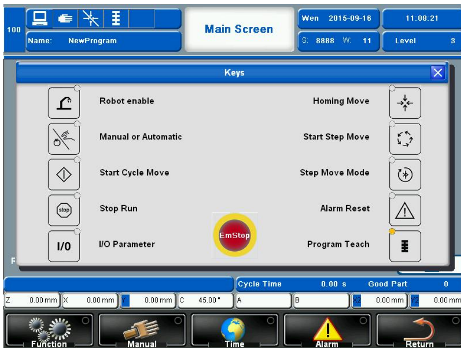
Fig.4-5: Main screen short-key function
