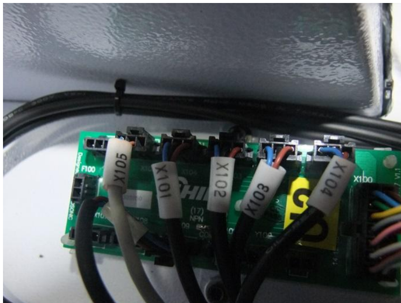
Fig.3-9: After exchanging X102 with X103
