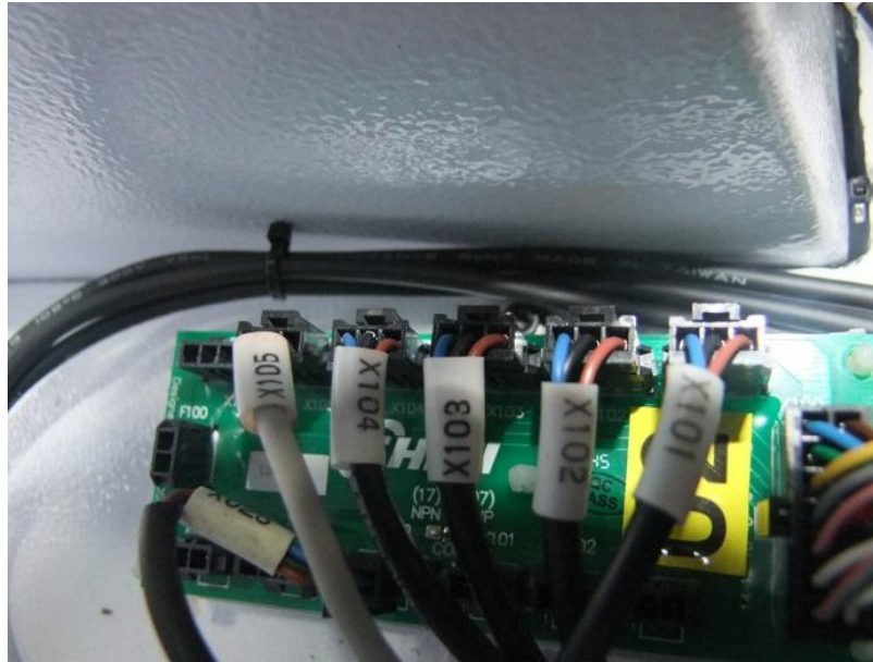
Fig.3-8: Before exchanging X102 with X103
