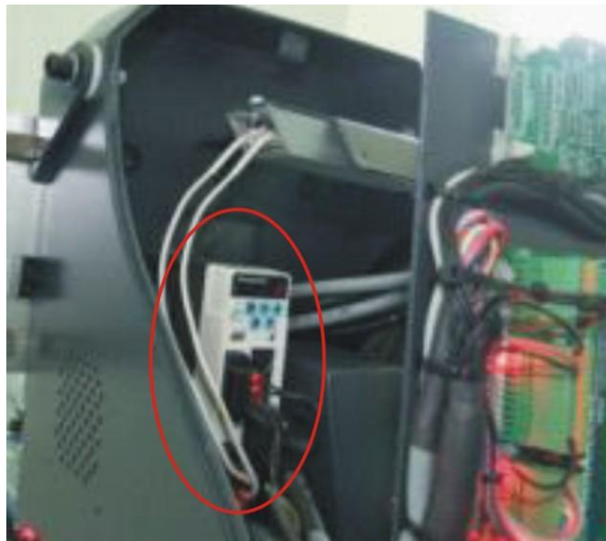
Fig.3-11: Traverse servo driver location
