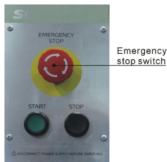
Picture 2-2: Emergency stop switch
