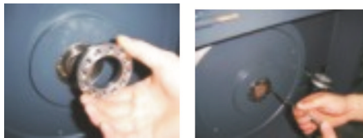
Picture 3-6: Installation of Belt and Belt Pulley 3
