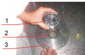
Picture 3-2: Installation of Bearing and Blade Rest
