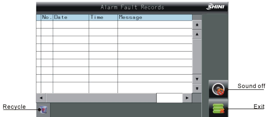
Picture 4-15: Alarm fault records
