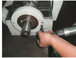
Picture 3-8: Installation of Rotating Blade and Fixed Blade 2
