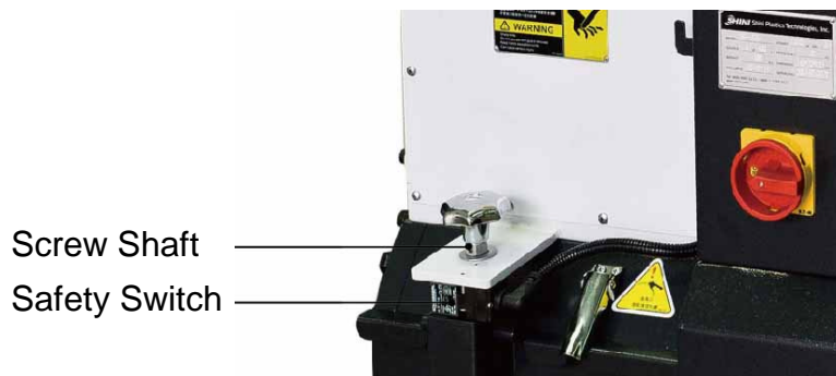
Picture 2-2: Safety Switch
