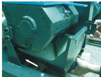
Picture 3-10: Installation of Material Storage Box 1
