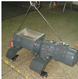
Picture 3-3: The Installation of Cutting Chamber
