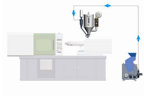
Picture 2-26: Loading With Blower
