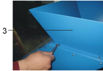
Picture 3-9: Installation of Feed Box Components 2
