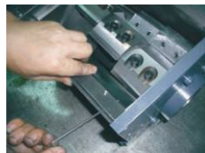
Picture 3-7: Installation of Rotating Blade and Fixed Blade 4
