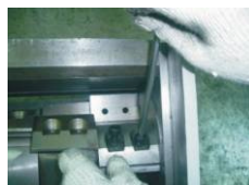
Picture 3-5: Installation of Rotating Blade and fixed Blade 2
