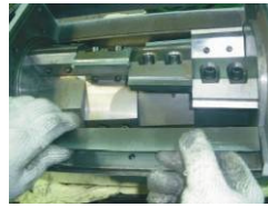
Picture 3-6: Installation of Rotating Blade and fixed Blade 3
