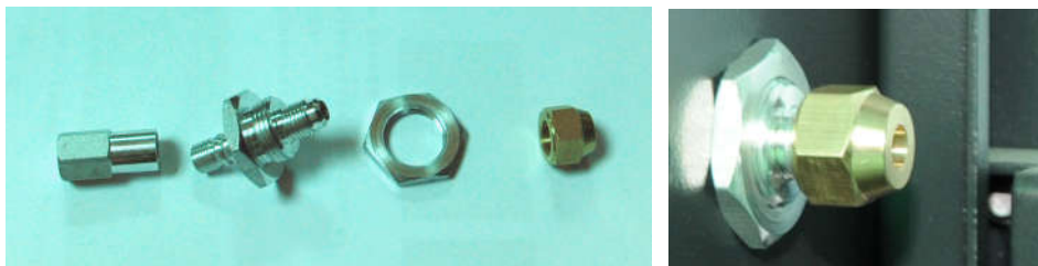
Picture 6-9: Copper Joint Assembly of Original Machine
