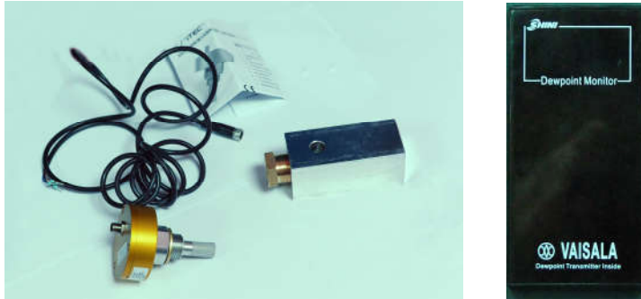
Picture 6-8: Parts of Dew-point Monitor
