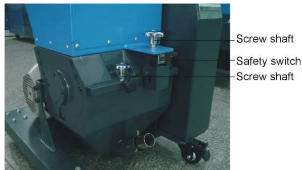
Picture 2-2: Safety System
