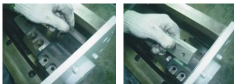
Picture 3-7: Installation of Rotating Blade and fixed Blade 1
