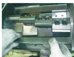
Picture 3-9: Installation of Rotating Blade and fixed Blade 3
