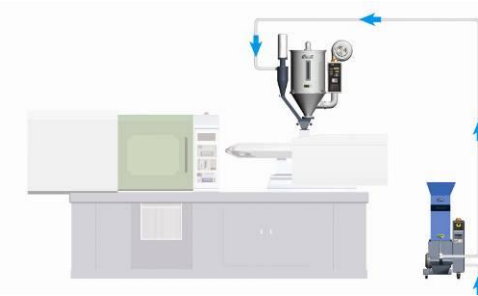
Picture 2-36: Loading With High Pressure Air
