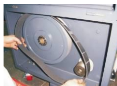
Picture 3-16: Installation of Belt and Belt Pulley 6
