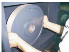
Picture 3-12: Installation of Belt and Belt Pulley 2
