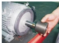
Picture 3-15: Installation of Belt and Belt Pulley 5
