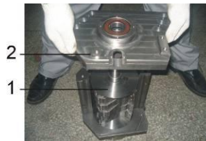
Picture 3-5: Installation of Bearing and Blade Rest 3
