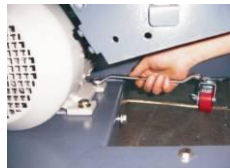
Picture 3-19: Installation of Belt and Belt Pulley 9
