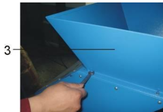
Picture 3-21: Installation of Feed Box and Feed Port 2
