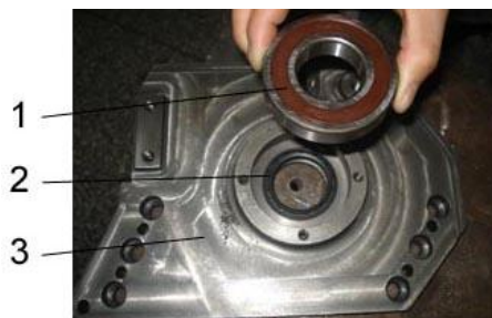
Picture 3-3: Installation of Bearing and Blade Rest 1
