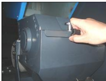
Picture 3-29: Installation of Material Collection Box 4
