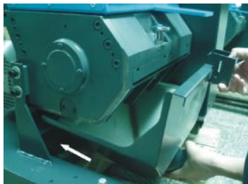
Picture 3-26: Installation of Material Collection Box 1
