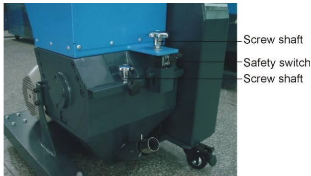
Picture 2-4: Safety System
