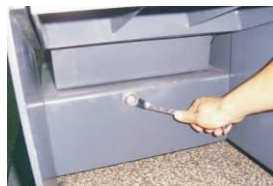
Picture 6-5: Adjustments of V Belts 1
