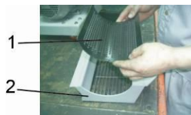
Picture 3-22: Installation of Screen and Screen Frame 1
