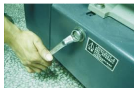
Picture 6-6: Adjustments of V Belts 2
