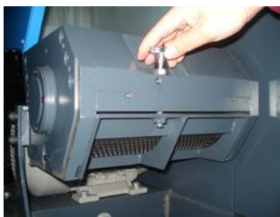
Picture 4-3: Open the Screen and Screen Frame 1
