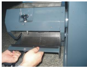
Picture 4-4: Open the Screen and Screen Frame 2
