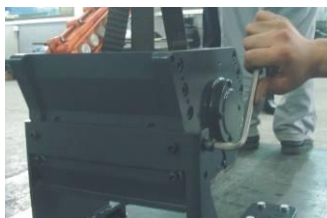
Picture 3-11: Installation of Belt and Belt Pulley 1
