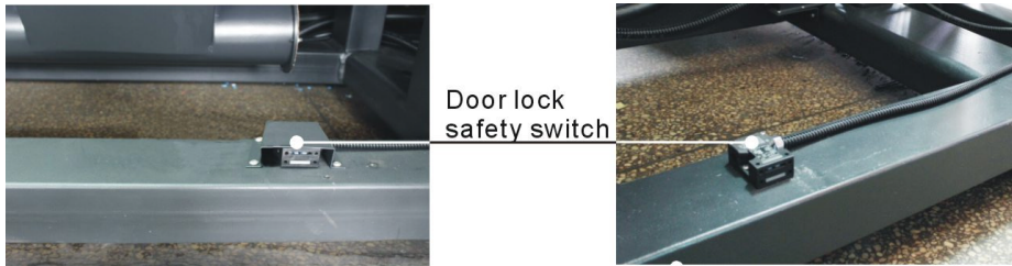
Picture 2-4: Safety Switch for Door Lock
