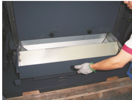
Picture 6-15: Installation of Storage Box, Screen and Screen Bracket 5
