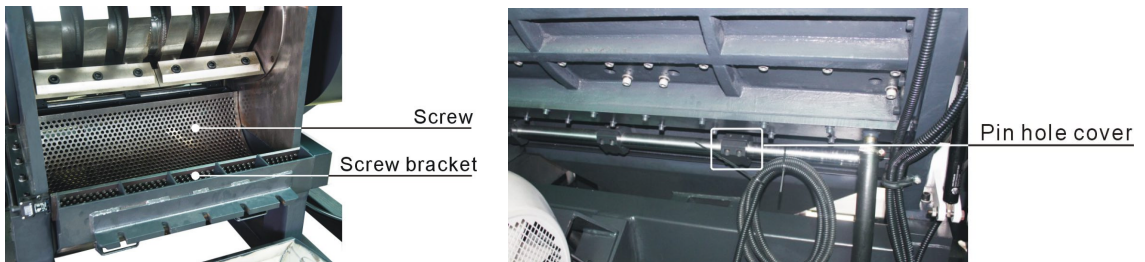
Picture 6-12: Installation of Storage Box, Screen and Screen Bracket 2
