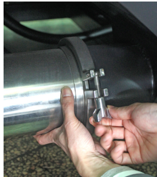
Picture 4-2: Loosen the Fast Pipe Clamp
