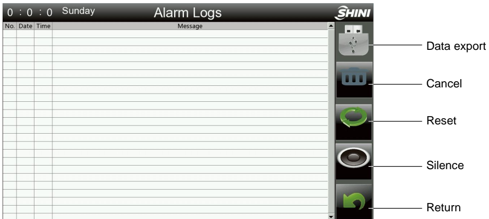
Picture 4-21: Alarm Fault Record
