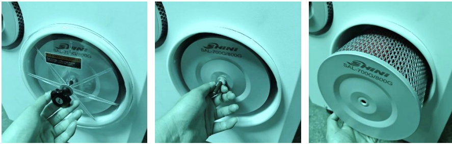
Picture 5-2: Filter Cleaning
