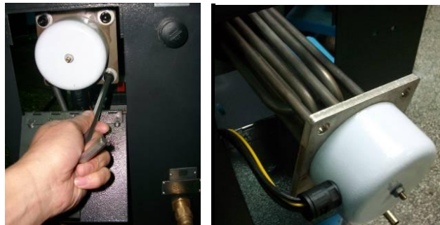
Picture 6-7: Pipe Heater 2
