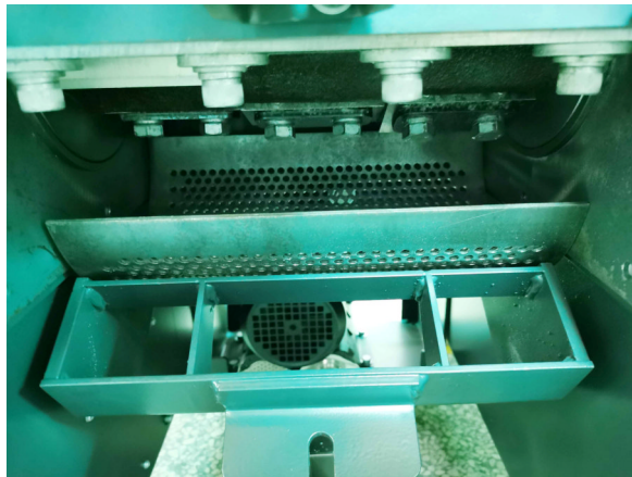
Pic. 6-8: Screen Installation
