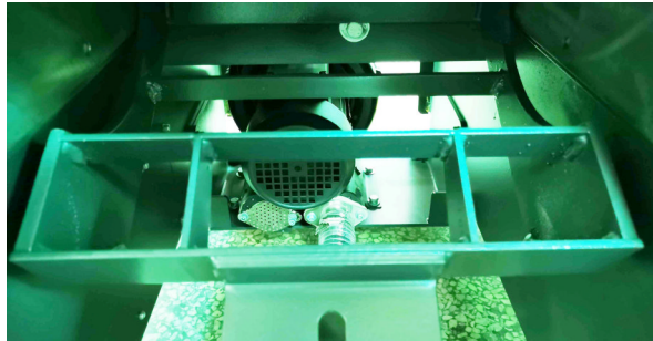
Pic. 6-7: Installation of Screen Bracket
