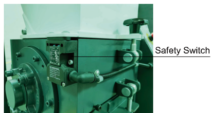
Pic. 2-3: Safety switch
