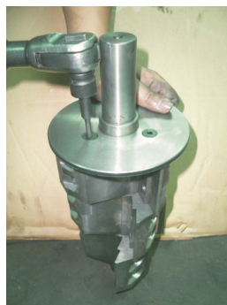
Pic. 6-2: Material Fender Installation
