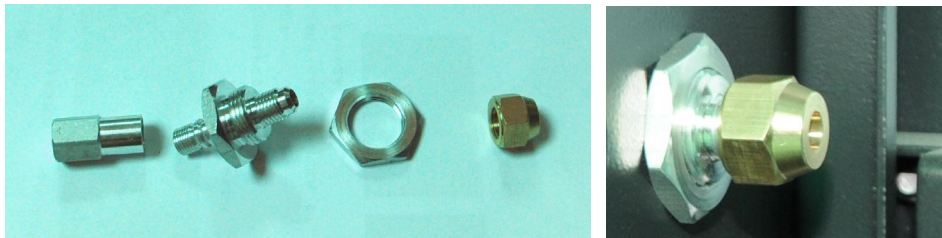
Picture 6-9: Copper Joint Assembly of Original Machine
