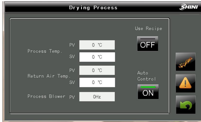
Picture 4-20: Drying Process Screen
