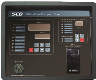
Dew-point Monitor (installed on machine)
