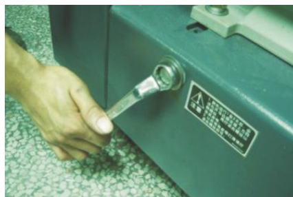
Picture 6-18: Adjustments of V Belts 2
