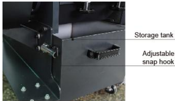
Picture 6-9: Collection Box Installation
