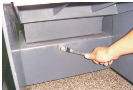
Picture 6-17: Adjustments of V Belts 1
