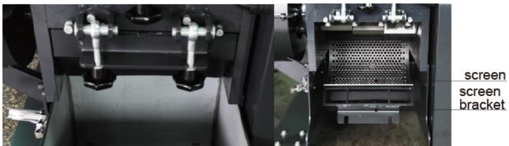
Picture 6-10: Open the Cutting Chamber
