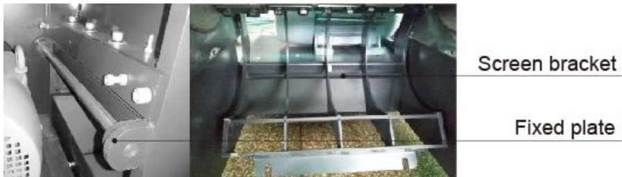
Picture 6-7: Installation of Screen Bracket
