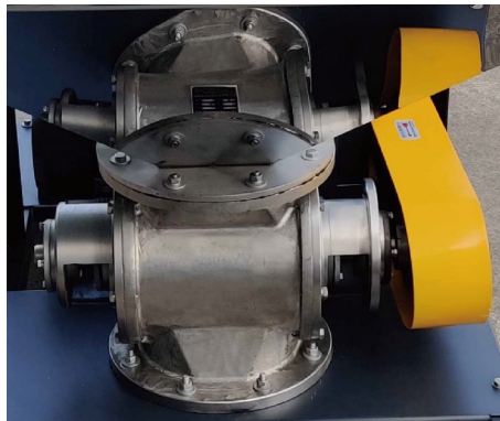
Picture 2-3: Rotary Valve
