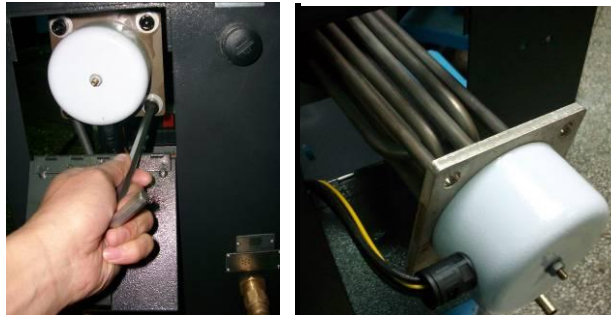
Picture 6-7: Pipe Heater 2
