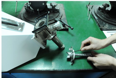
Picture 4-2: Replace Dosing Screws
