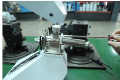
Picture 4-2: Replace Dosing Screws
