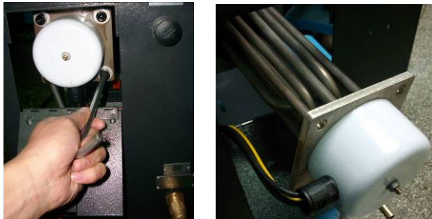
Picture 6-4: Heater Pipe 2
