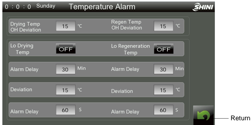
Picture 4-20: System Alarm Setting
