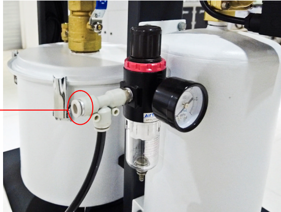
Fig. 3-2: Compressed Air Connecting Point
