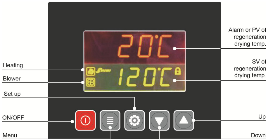
Picture 4-1: Control Panel
