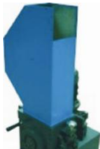
Picture 3-10: Installation of Feed Box, Feed Throat and Storage Box 1
