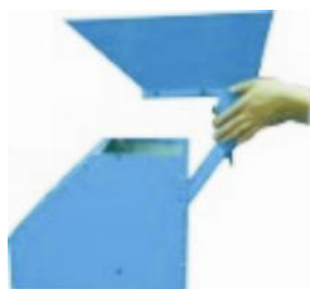
Picture 3-11: Installation of Feed Box, Feed Throat and Storage Box 2
