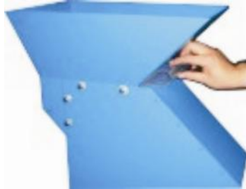
Picture 3-12: Installation of Feed Box, Feed Throat and Storage Box 3
