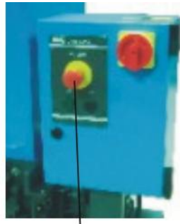
Emergency stop switch
