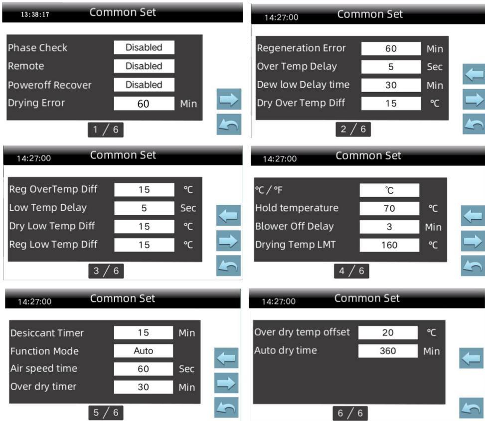
Picture 4-40: Project Setting - Comm. Setting Screen ( Adaptive mode )
