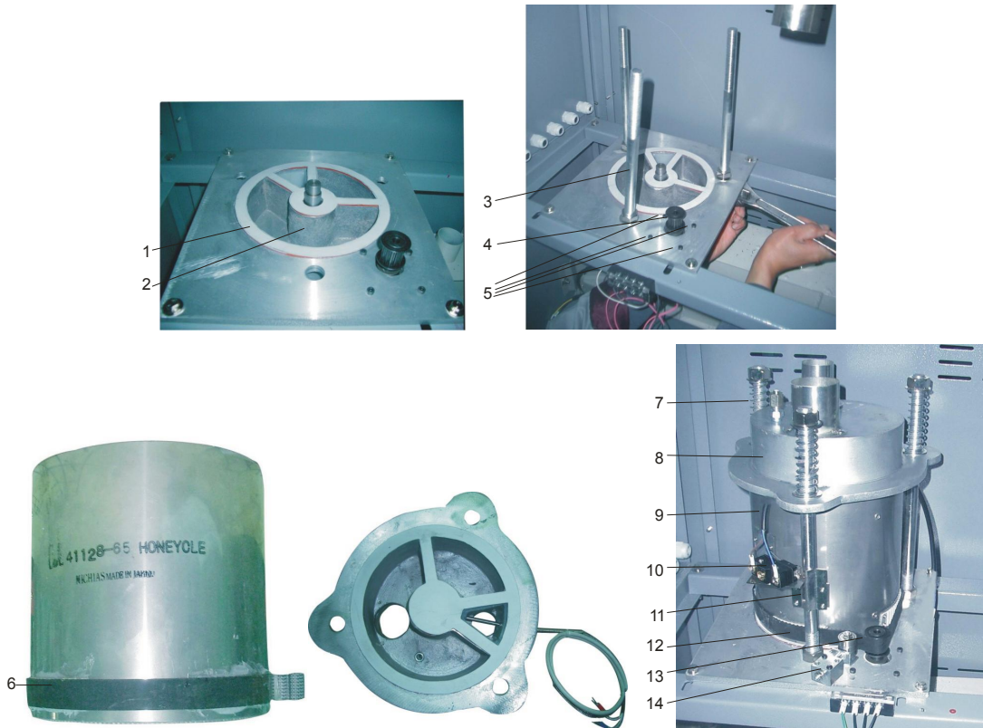
Picture 6-3: Installation of The Rotor
