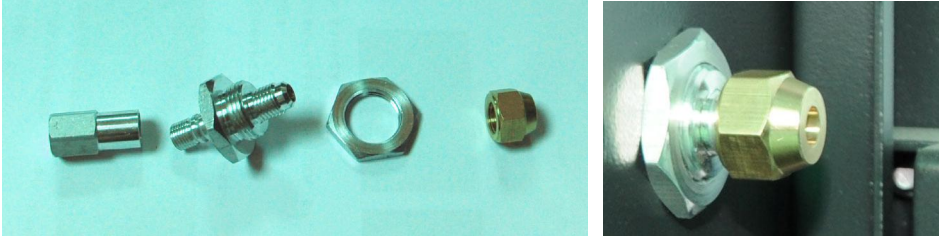
Picture 6-7: Copper Joint Assembly of Original Machine
