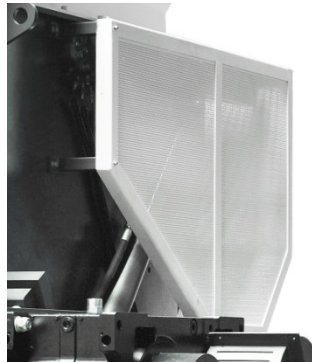
Picture 6-2: Installation of the Shield
