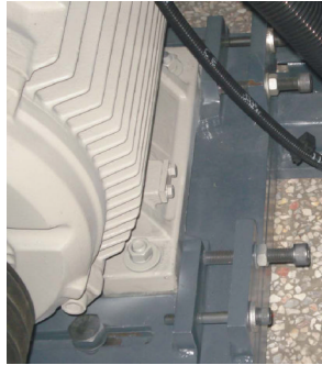
Picture 6-13: Adjustment of V-belt
