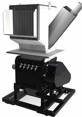
Picture 2-11: Material Side Feed Pipe
