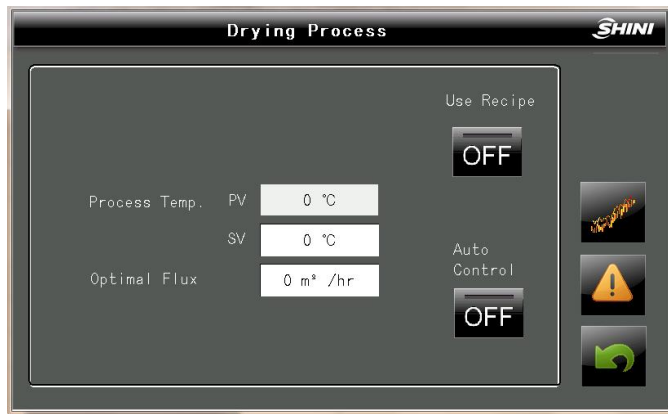
Picture 4-14: Drying Process Screen
