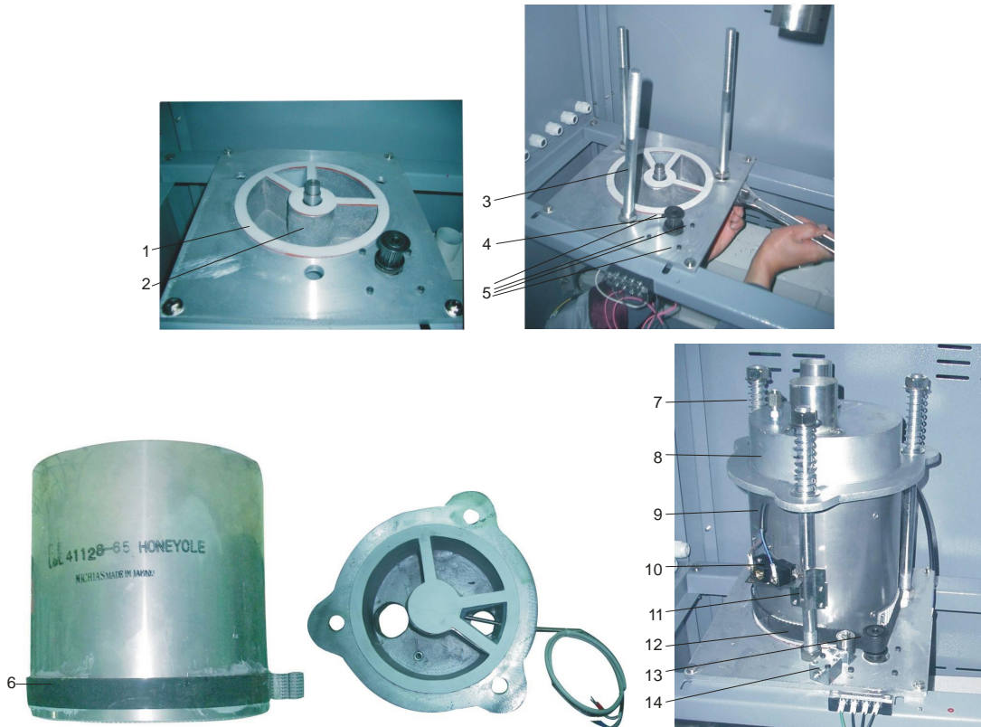
Picture 6-8: Installation of the rotor
