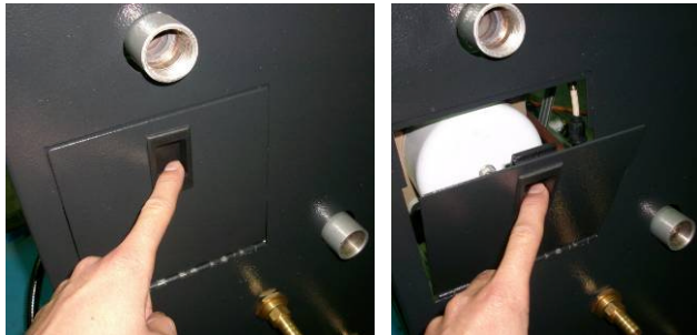
Picture 6-6: Pipe Heater 1
