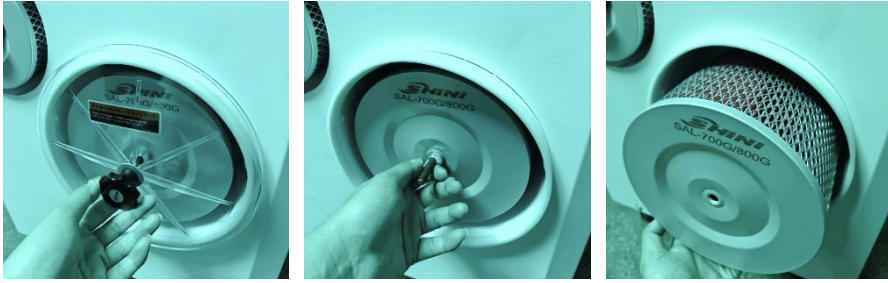
Picture 6-2: Filter Cleaning
