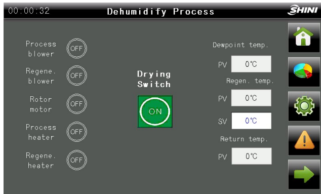
Picture 4-15: Dehumidify Process Screen
