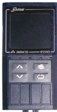
Picture 4-1: Temp. Controller
