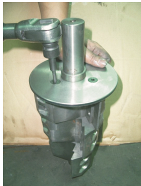
Picture 3-4: Installation of the Flap
