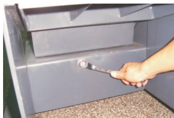
Picture 6-3: Adjust the V-belt 1
