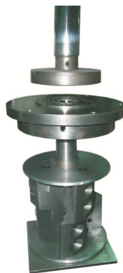
Picture 3-5: Installation of Bearing Block and Bearing
