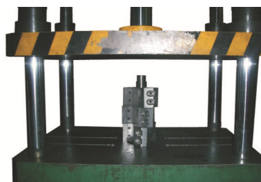
Picture 3-3: Installation of Blade Rest Shaft
