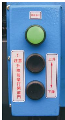
Picture 4-3: Electrical handspike operational button
