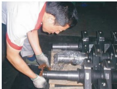
Picture 3-6: Installation of Bearing and Blade Rest
