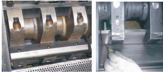
Picture 3-7: Installation of Fixed Blades and Rotating
