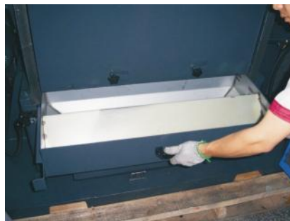
Picture 3-14: Installation of Screen, Screen Bracket and Storage Box 5
