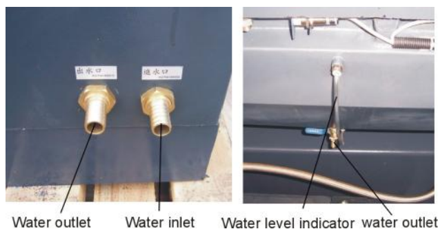
Picture 3-16: Connection to Cooling Water
