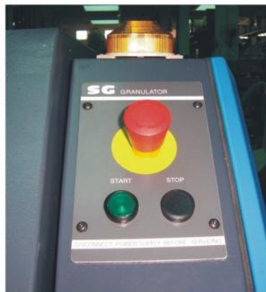
Start/stop button and emergency stop button
