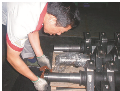
Picture 6-5: Installation of Bearing and Blade Rest
