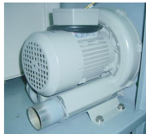
Picture 6-3: Installation of Blowers
