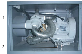
Picture 6-4: Conveying Blower
