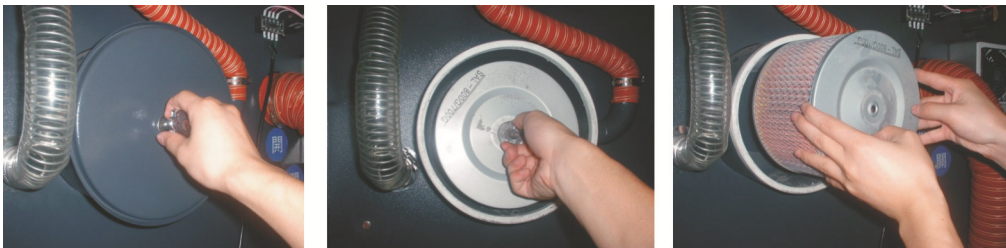
Picture 6-3: Dust Collecting Barrel Cleanout
