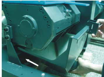
Picture 3-10: Installation of Material Storage Box 1
