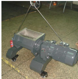
Picture 3-3: The Installation of Cutting Chamber
