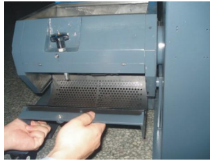
Picture 4-4: Open the Screen Bracket and Screen 2
