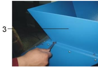
Picture 3-9: Installation of Feed Box Components 2
