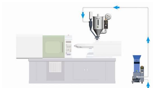
Picture 2-25: Loading With High Pressure Air
