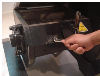
Picture 4-3: Open the Screen and Screen Bracket 1
