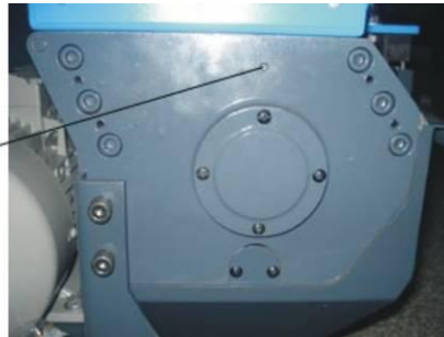
Picture 6-5: Dust Collection Chamber Cleaning
