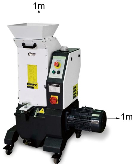
Picture 3-1: Installation Layout
