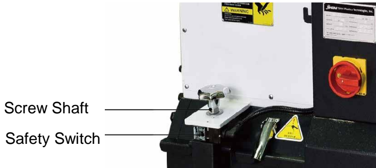
Picture 2-4: Safety System
