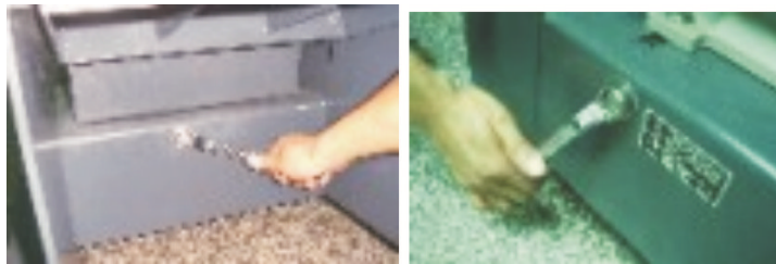
Picture 6-5: Adjust the V-belt
