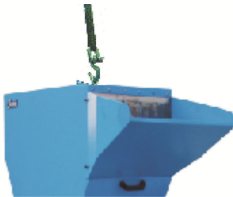
Picture 3-11: Installation of Screen, Screen Frame and Storage Bin 1
