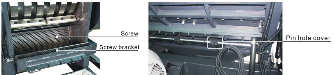
Picture 6-12: Installation of Storage Box, Screen and Screen Bracket 2
