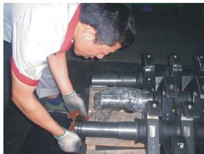
Picture 6-6: Bearing and Blade Rest Installation Drawing
