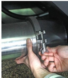
Picture 4-2: Loosen the Fast Pipe Clamp
