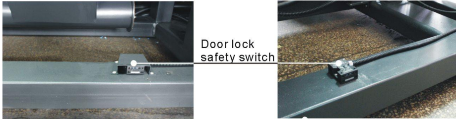
Picture 2-4: Safety Switch for Door Lock
