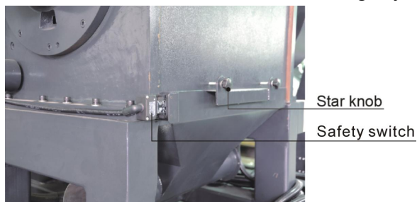
Picture 6-16: Installation of Storage Box, Screen and Screen Bracket 6
