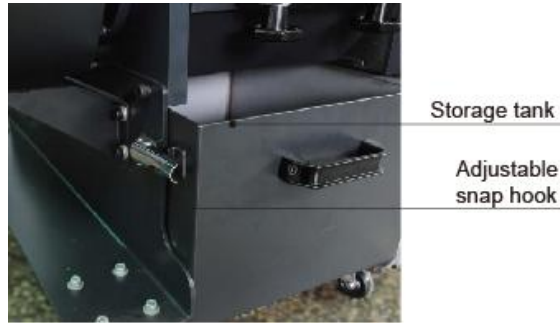
Picture 6-9: Collection Box Installation
