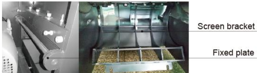
Picture 6-7: Installation of Screen Bracket
